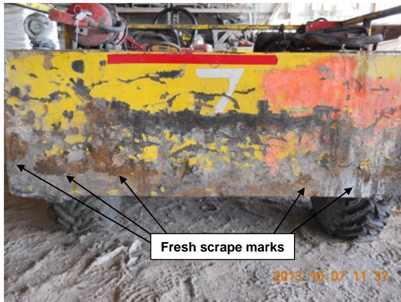
Rear bumper of company No. 7 battery-powered personnel carrier
