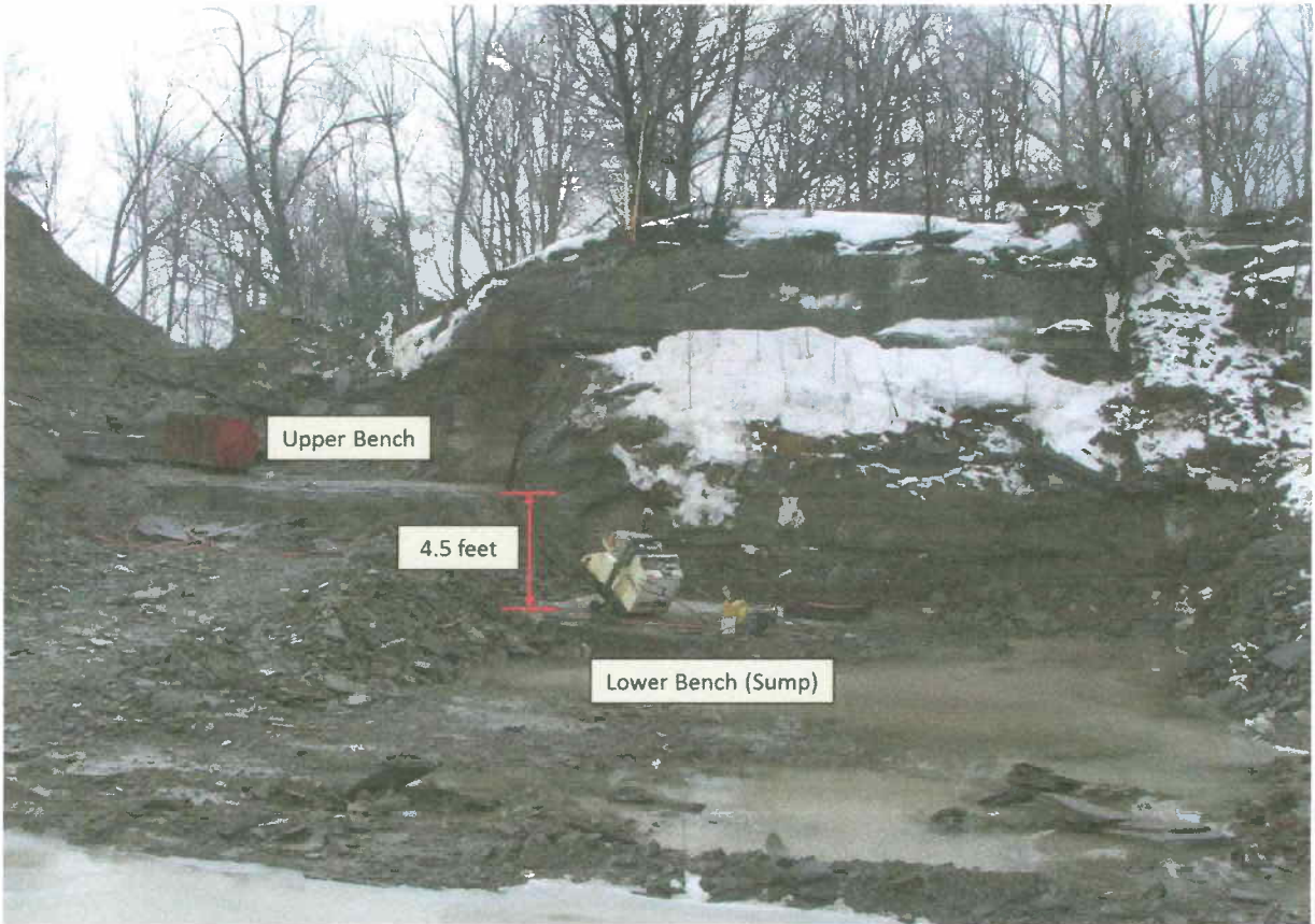
Figure 1 – Victim was sawing stone blocks on the upper bench when he fell to the lower bench below (sump area) and the saw fell on top of him.
