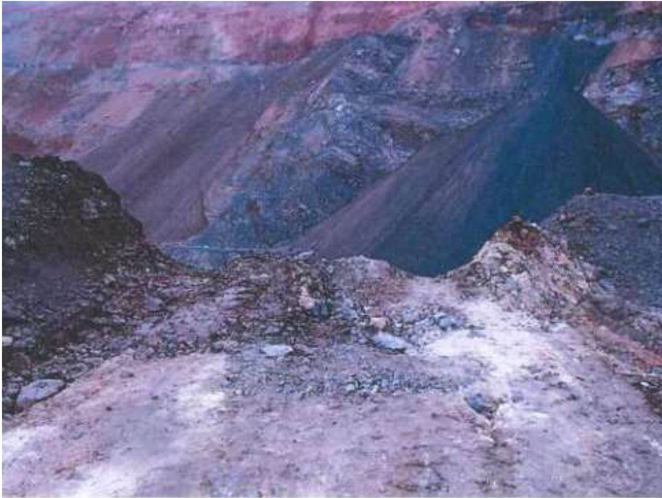
Dump Site Berm Where Haul Truck Travelled Thru
