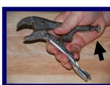
**Contact Stress/Pressure Points** - using a tool with a too short handle
